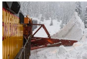
A spreader with 30-foot split wings pushes snow away from the main line at Eder, California.
