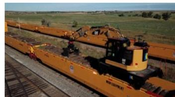
The new Maintenance of Way Tie Pickup work equipment follows a tie gang in Western Nebraska.
