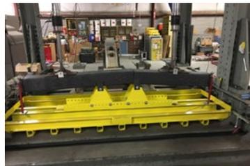
Engineering is testing several types of composite ties in-house, using this machine to determine which perform best.
