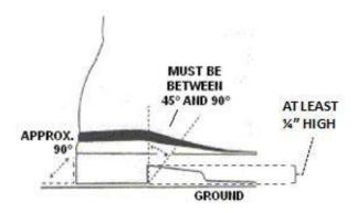
Defined heel - 1/2" deeper than the rest of the sole when new. At no time should that measurement be less than 1/4".
